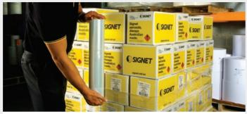
Allow the film to unwind freely as you walk towards one of the corners of the pallet
