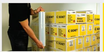
After stretching the film, step around the corner with the tension still applied to prevent puncturing or tearing. Then release and let the film unwind freely.
