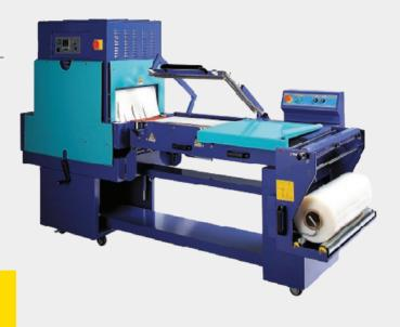
Sealing Area: Max Film: Power Supply: 400mm (W)  $\times$  550mm (L)  $\times$  150mm (H) 610mm × 250mm Diameter 415V, 50HZ, 3-phase
