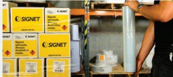
Stretch the film by 30-50%, feeling the tension, before wrapping it around the corner.
