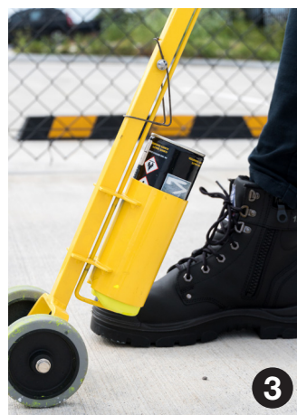
3 Ensure can is securely loaded and is now at the back of Spotting Handle.
